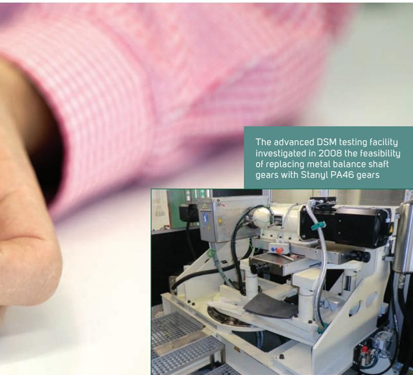
The advanced DSM testing facility investigated in 2008 the feasibility of replacing metal balance shaft gears with Stanyl PA46 gears
