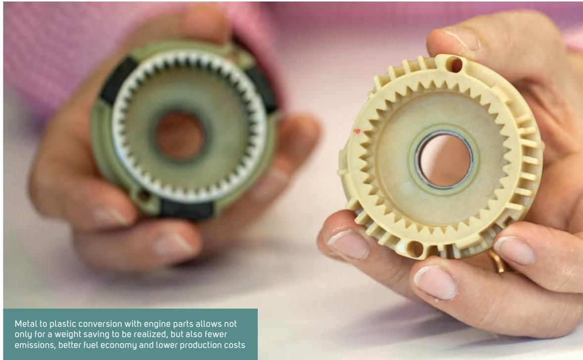
Metal to plastic conversion with engine parts allows not only for a weight saving to be realized, but also fewer emissions, better fuel economy and lower production costs
